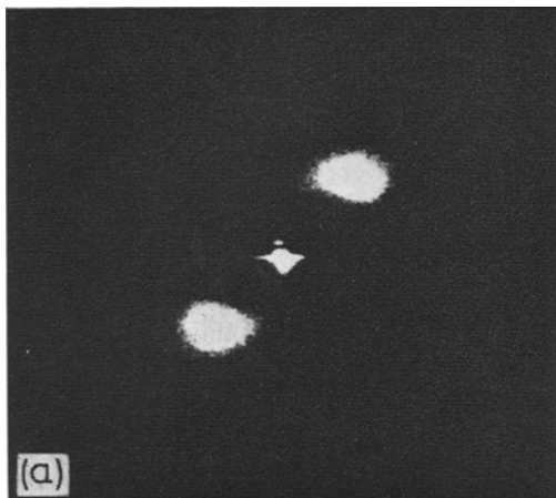
Figure 27 Low angle X-ray diffraction patterns of single texture specimens annealed at 95°C showing large reversible change in spacing. (a) at room temperature (b) at 95°C. (The sharp cut-off of the reflection at small angles is not due to an obstruction, it is a genuine feature of the pattern).
